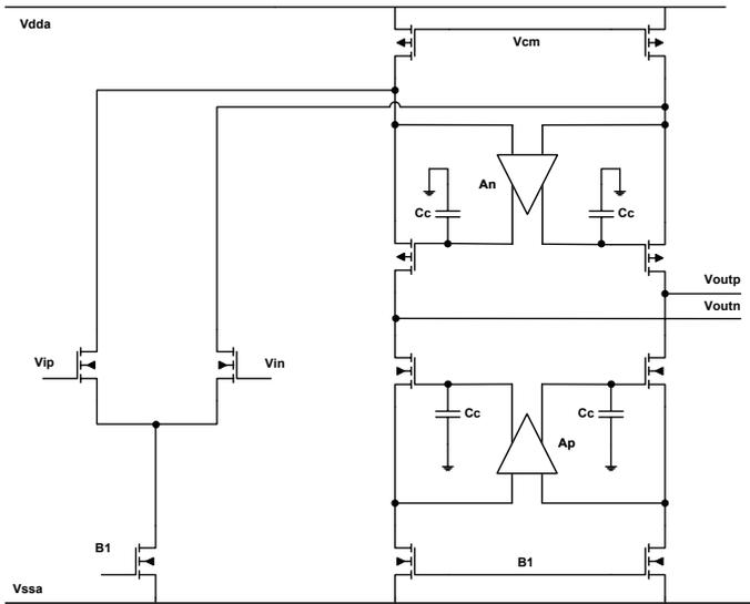
Fig. 2. OTA circuit with fully differential gain enhancement.
