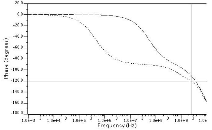
Fig. 6. Open loop Bodeplot with and without gain enhancement, showing the phase.
