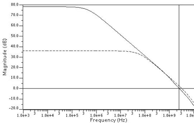
Fig. 5. Open loop Bodeplot with and without gain enhancement, showing the amplitude.
