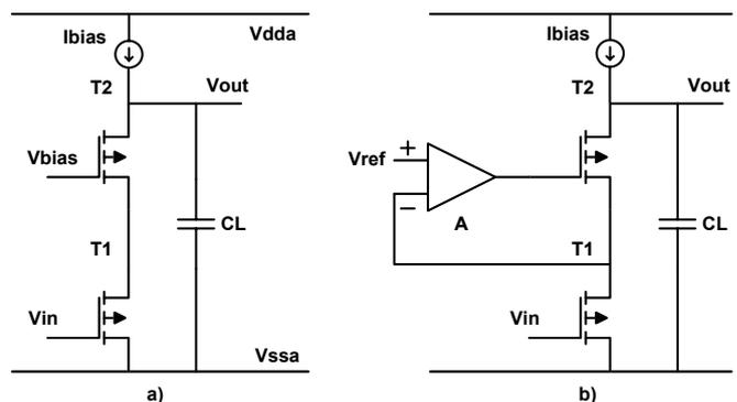
Fig. 1. (a) Regular cascode circuit. (b) Active cascode circuit.
