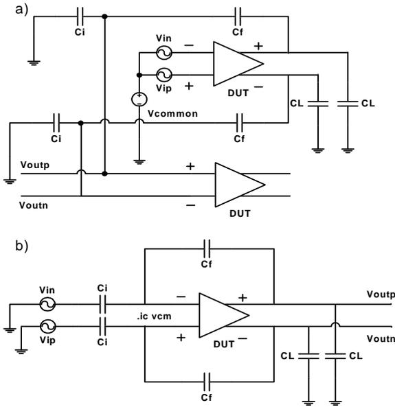
Fig. 4. (a) Open loop testbench used to simulate the frequency response. (b) Closed loop testbench used to simulate settling.
