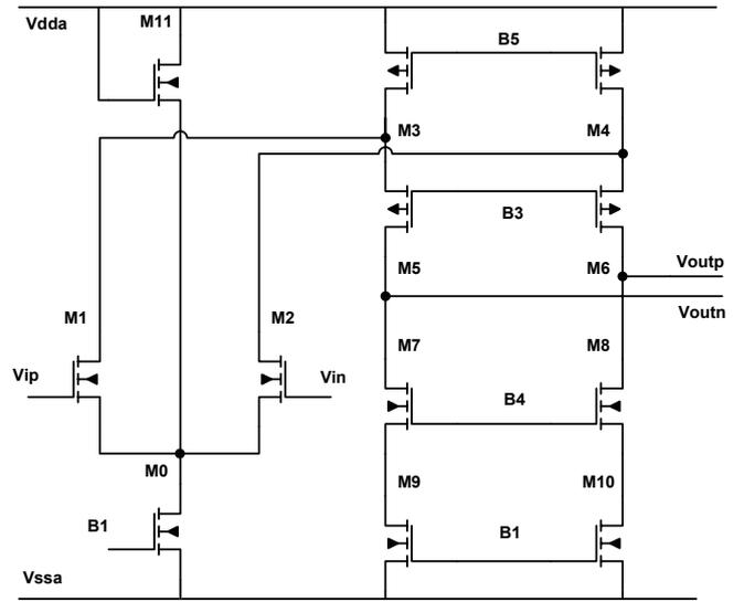
Fig. 3. Fully differential supplemental OTA .
